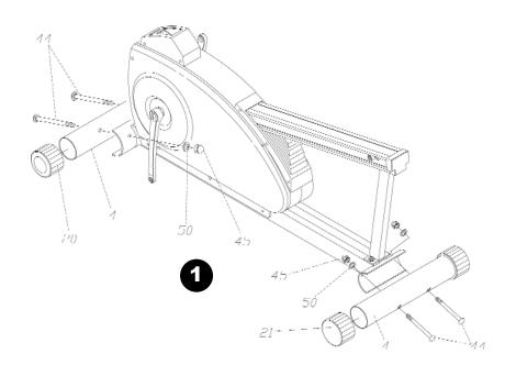
**1.** Attach foot tubes (4) to the frame by using the carriage bolts (44), flat washers (50) and cap nuts (45) provided. Make sure the foot tube with wheels is assembled onto the front of the unit.
